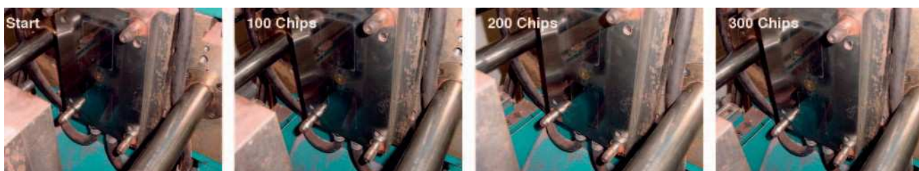
Fig. 2. No plate-out during the RadGlo test of the RPC Series: 2 % in 5 kg PE-HD (300 chips)
