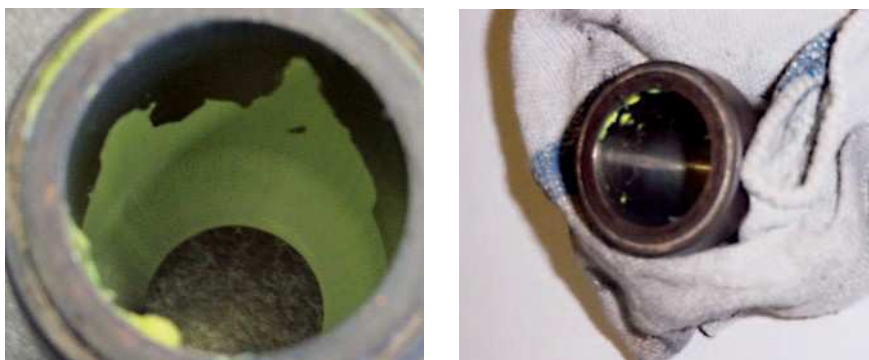
Fig. 3. Plate-out on the conical extruder sleeve when extruding with RadGlo EA10 (left) and RadGlo RPC10 (right)
